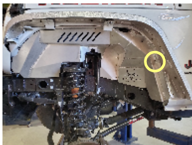
Bottom Rear Bolt is Missing in the Photo
