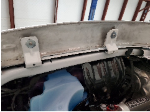
Bolts installed in Factory Flare Braces
