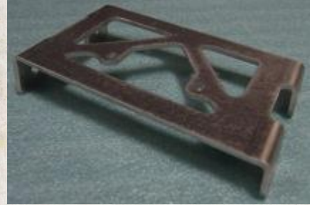
Battery Hold Down Riser
